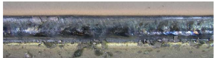
Fig. 2 Bead Appearance of Slag Removed
