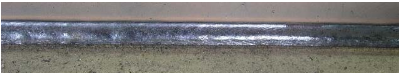
Fig. 2 Bead appearance of slag removed
