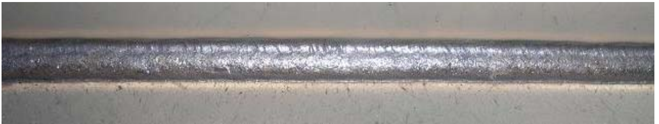
Fig. 1 Bead appearance of slag covered
