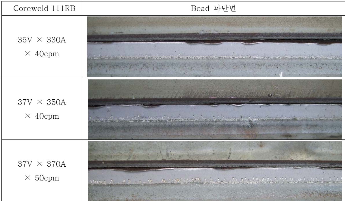
Fig. 4 Robust anti blowhole property of Test Specimen
