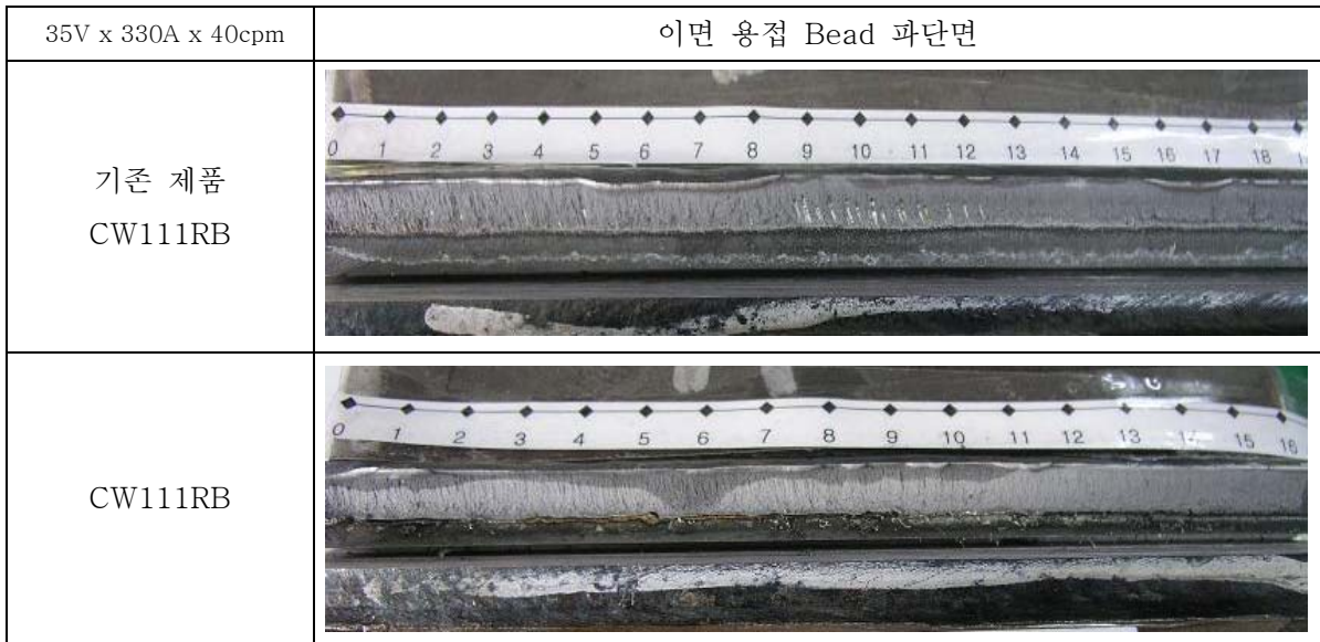
Fig. 5 Blowhole state of Rupture Test Specimen
